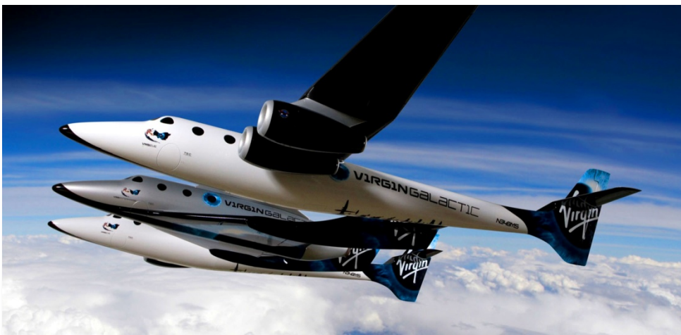
Virgin Galactic has unveiled a SpaceShipTwo (SS2) design, created by Scaled Composites, that harks back to the NASA/USAF Boeing X-20 Dyna-Soar glider of the 1960s, while Scaled's carrier aircraft, White Knight II (WK2) has been given a twin-fuselage configuration.
